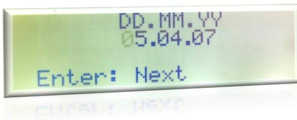
The date is set starting from the leftmost digit. The digit set by the “up” and “down” direction buttons is saved when the “enter” button is pressed and the cursor moves to the next digit.
