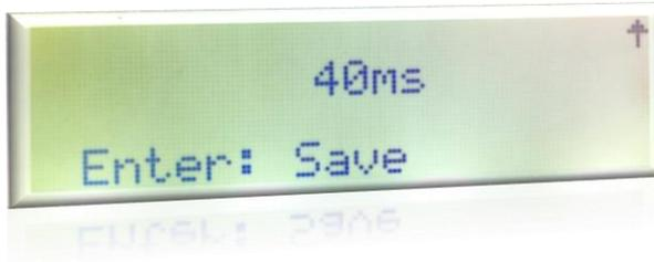
The detection time is set between 40 and 800 ms in 40 ms steps. The value is changed by the “up” and “down” direction buttons. The value is saved when the “enter” button is pressed.
