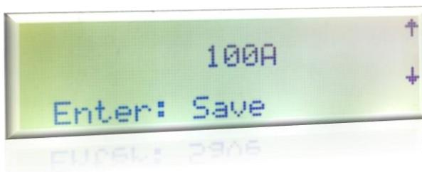
The phase current threshold value is set in this page. The desired value is set between 50 and 1000A with 50A steps with the “up” and “down” direction buttons. Pressing the “enter” button, the value is saved and page is returned to the settings page.
