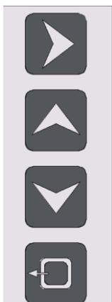
**Enter:** It logs in the page where the cursor is located. It saves the set parameters. In the pages where more than one parameters are set, the page immediately goes to the next parameter.
