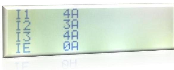
The "Measurements" page displays the current values of the network. When the “Esc” button is pressed, the menu page opens.
