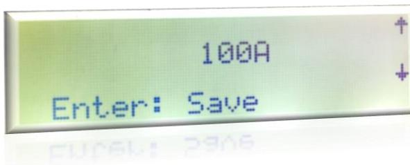
The earth current threshold value is set in this page. The desired value is set between 20 and 200A with 20A steps with the “up” and “down” direction buttons. Pressing the “enter” button, the value is saved and the page returns to the settings page.
