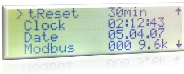
In this page, the fault current values and the time required for the fault condition to occur, auto reset time, time-date settings and Modbus parameters can be set.
