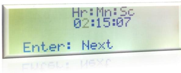
The time is set starting from the leftmost digit. The digit set by the “up” and “down” direction buttons is saved when the “enter” button is pressed and the cursor moves to the next digit.
